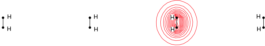
Figure 3.15: Four H 2 molecules at large distances. The contour plot of the bonding HF orbital of one H 2 molecule is shown.
