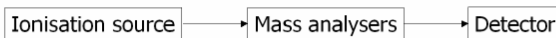
Figure 4. The basic components of a mass spectrometer. The collision cell is typically not an analyzer, and normally located between mass analyzers or directly after.
