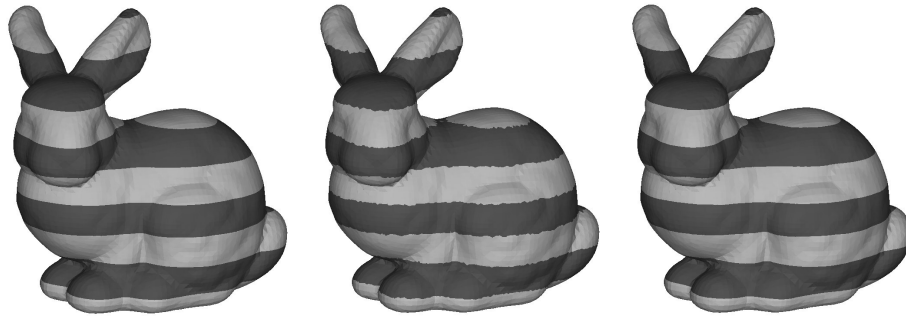
Figure 7.12: Image denoising with level set representation of the surface. From left to right: original image, noisy image, image after 5 timesteps. [0, 4] \times [0, 4] \times [0, 4] , grid with 192.000 grid points, grid size h = 0.039 at the surface and timestep \Delta t = 0.001 .
