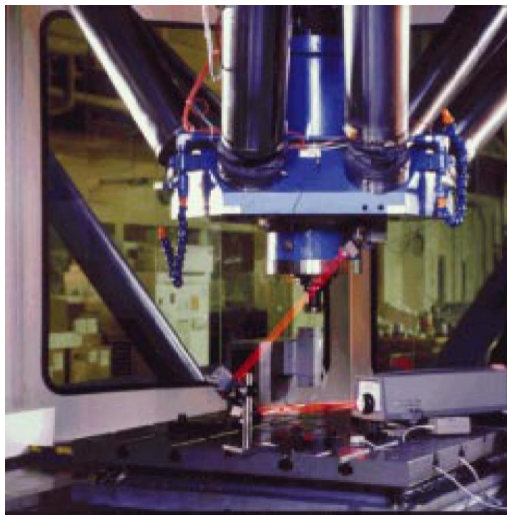
Fig. 2.15: Special set-up to measure the relative strut lengths error [Wav98]
