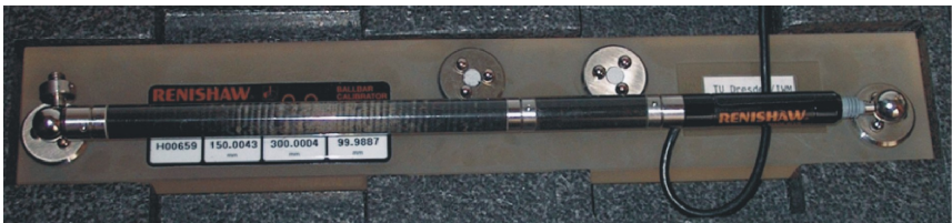
Fig. 4.10: Double-Ball-Bar and Zerodur © calibration unit
