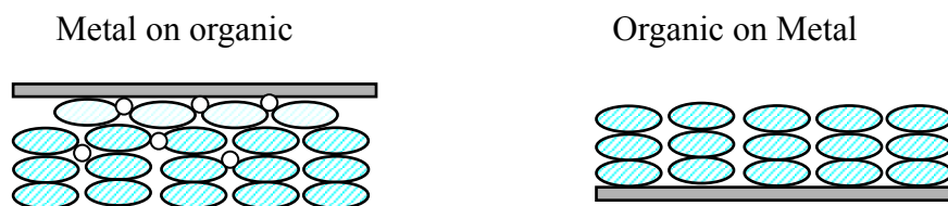
Fig. 5.11. Schematic diagrams of (left) an organic/metal interface and (right) a metal/organic interface.
