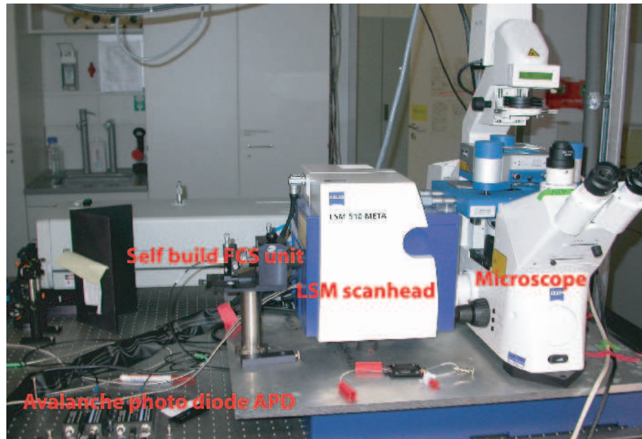
Figure 2.16: The actual confocal FCS setup applied to Min proteins mobility measurements. See "Optical Setup" in appendix A for details.
