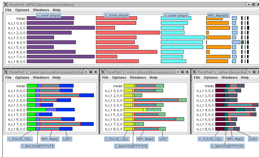
Figure 2.21: ParaProf’s two-level displays for phase-based profiles. In the top window the three phases are shown in a compound way. The phases correspond to three main functions of an iterative solver software [BHdW + 95]. Some operations appearing outside of explicit phases can be shown separately. The three phase-specific displays below present the details for the phases separately for all processes. Smart highlighting allows the identification of common function calls over all phases. (Taken from [MSM05].)
