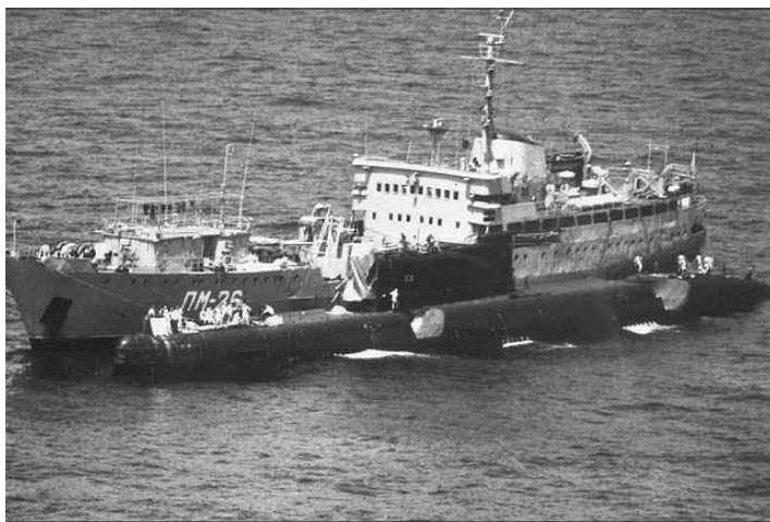
A Juliett-class submarine being repaired at sea
