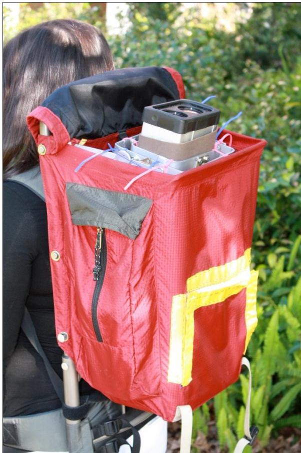
Figure 25. Portable LiDAR unit in the backpack frame.
