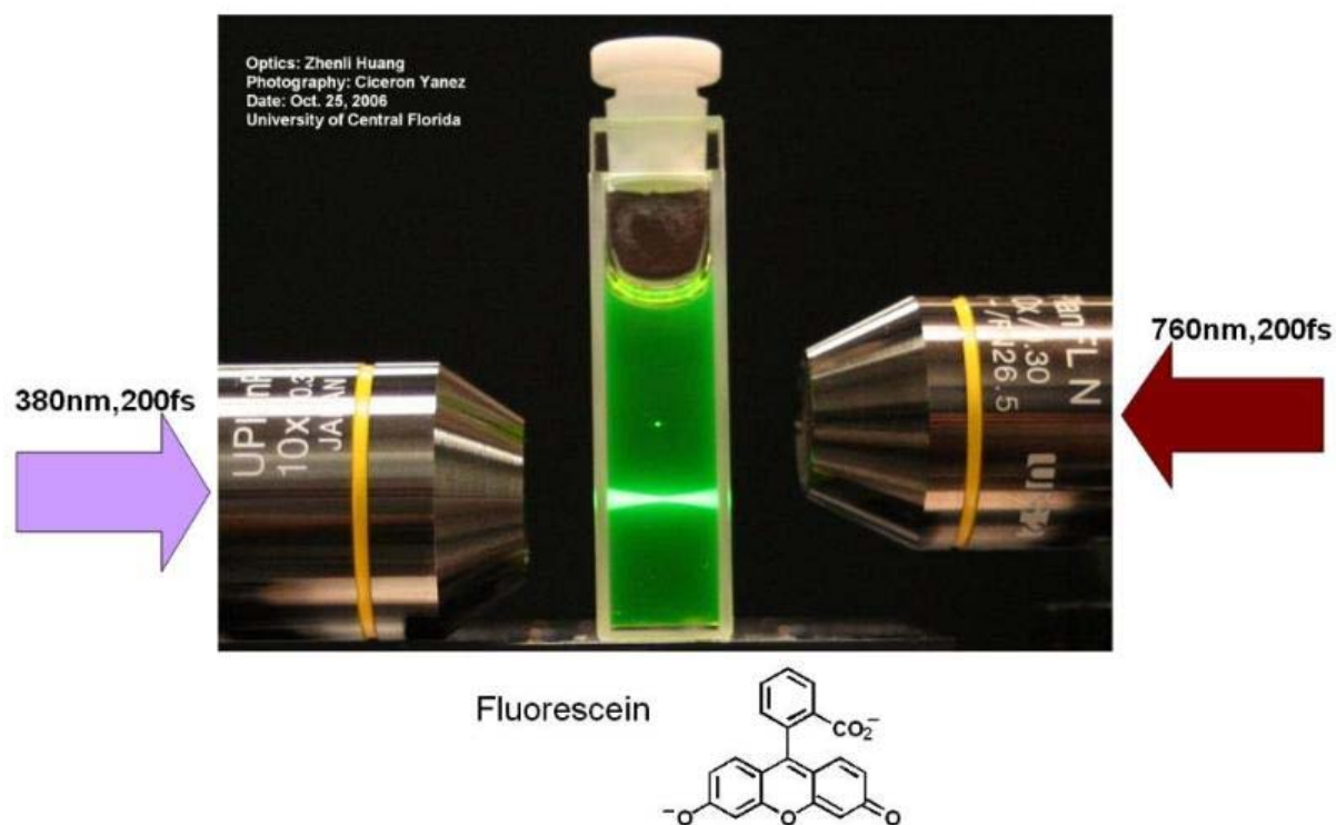
Figure 2. Demonstration of excitation under conventional one-photon absorption (lower) in a comparison with two-photon absorption (upper). Note: in case of 2PA, the excitation is localized in a spot smaller than the fluorescent spot seen in the picture. The solution contains 5 \cdot 10^{-5} M of fluorescein. Other experimental conditions can found on the research group website. 4
