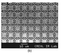
Fig. 5. Completed polyimide FSS: (a) flexible 10 cm (4 in.) wafer fully populated and (b) elements intact on flexible substrate after polyimide backing removal.
