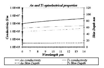
Fig. 4. Spectral conductivity and skin depth derived from optical constants measured with IR-VASE ellipsometer.
