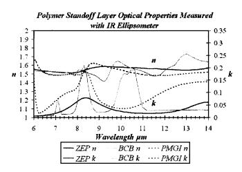
Fig. 2. Mid-IR optical properties of polymers.
