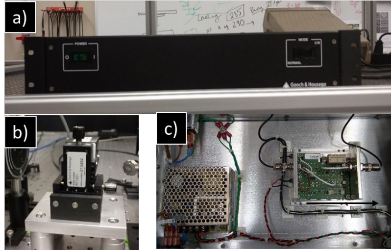
Figure 17. (a). In-house voltage divider box whose major components are a fan and a RF driver, (b) the AOM was placed in the beam path, and (c) Inside of the line divider box.
