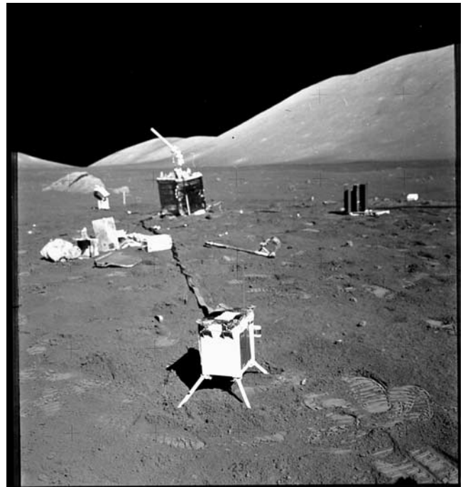
Figure 6. Apollo 17 Lunar Surface Experiments Package. The box in the foreground is the Lunar Ejecta And Meteorites (LEAM) Experiment. NASA photograph AS17-134-20500, National Space Science Data Center.
