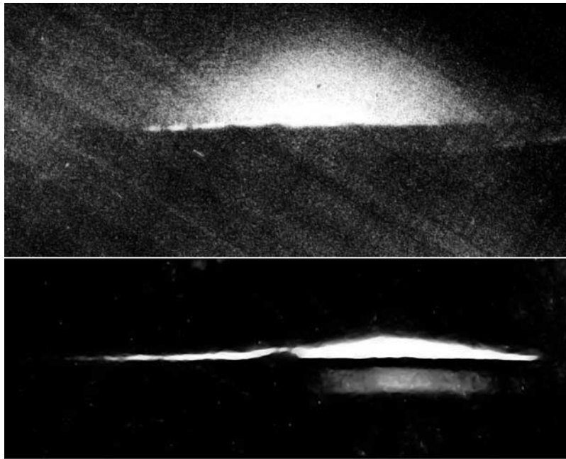
Figure 5. Contrast enhanced and low-pass-filtered images of lunar horizon glow from (top) Surveyor 6 and (bottom) Surveyor 7. The apparent gap between the horizon glow and the lunar surface noted by Rennilson and Criswell [1974] can also be explained by forward scattering of light from the cloud itself to illuminate part of the lunar surface between the horizon and the spacecraft. Photographs from National Space Science Data Center.
