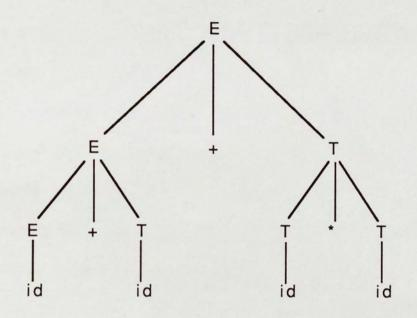
Figure 3.8. A Parse Tree Whose Height is Proportional to the Logarithm of the Length of the String Being Parsed.
