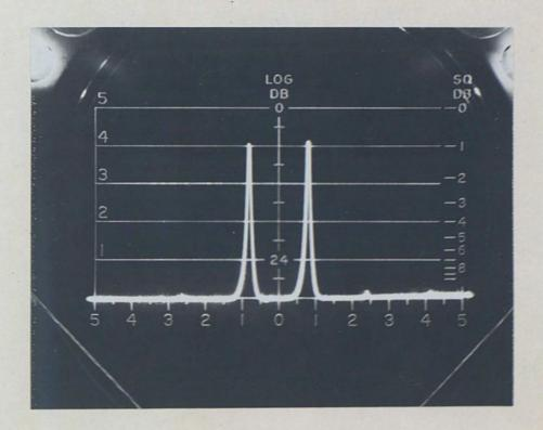
Figure 6. The cos a and cos b Signals Attenuated 6 dB from the Level of Figure 4.
