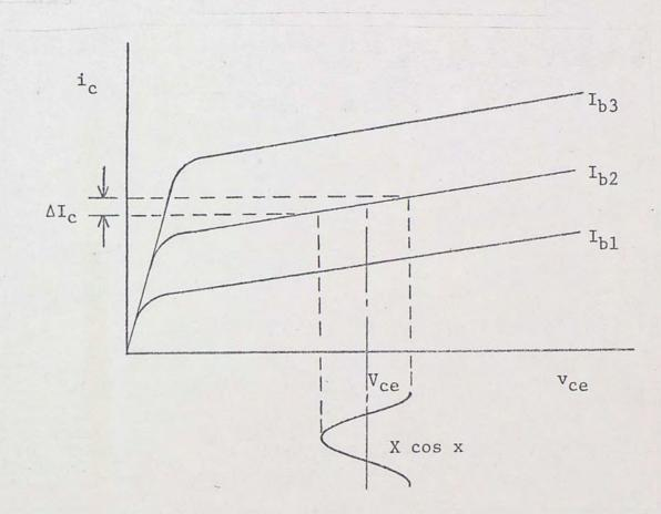
As can be seen, the presence of the signal, X cos x, introduced at the collector of a transistor will modulate the output current. Indeed. this is the method used in high level amplitude modulation. The modulation effect can be seen to be greater if the transistor is operated in the saturation region.
