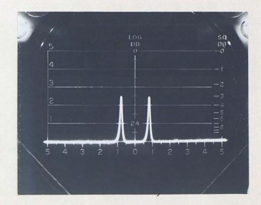
Figure 7. The cos a and cos b Signals Attenuated 12 dB from the Level of Figure 4.
