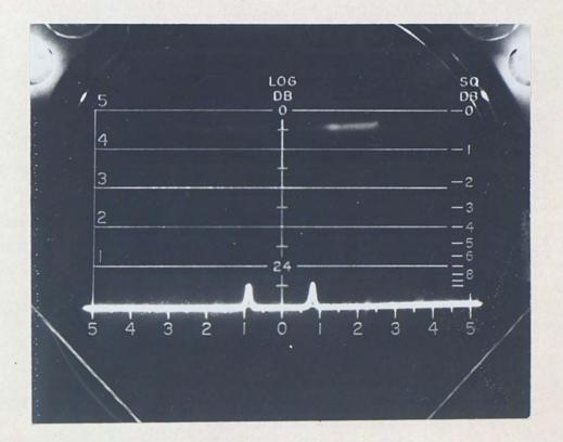
Figure 9. The cos a and cos b Signals Attenuated 24 dB from the Level of Figure 4.
