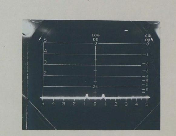
Figure 10. The cos a and cos b Signals Attenuated 30 dB from the Level of Figure 4.
