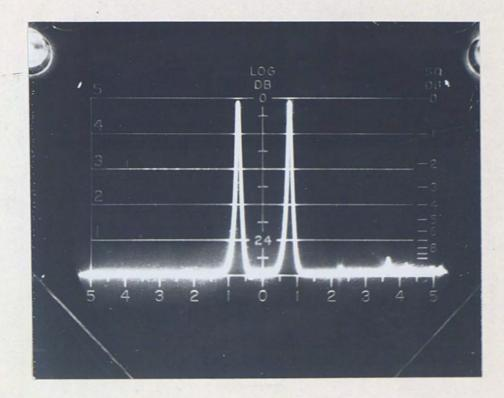
Figure 4. Output Power Spectrum Showing the cos a 105.6 MHZ (Right of Center) and the cos b 106.5 MHZ (Left of Center) Signals and the IM3 cos(2a-b) 104.7 MHZ (at 2.4 on the Horizontal Graticule) and the IM5 cos(3a-2b) 103.8 MHZ (at 3.6 on the Horizontal Graticule. This is from the Push-Pull Amplifier Output.
