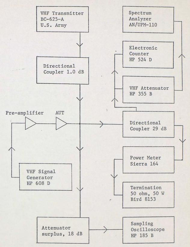
Figure 3. Test Set-up for Measuring Intermodulation Distortion
