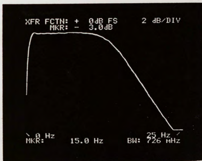
Figure 18. Frequency Response for Channel 1 (0-25 Hz).
