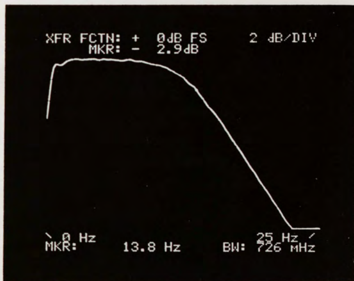
Figure 20. Frequency Response for Channel 2 (0-25 Hz).
