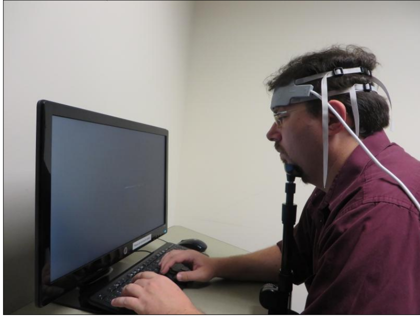
Figure 8: Participant doing the categorization task on the computer while wearing an fNIR sensor pad
