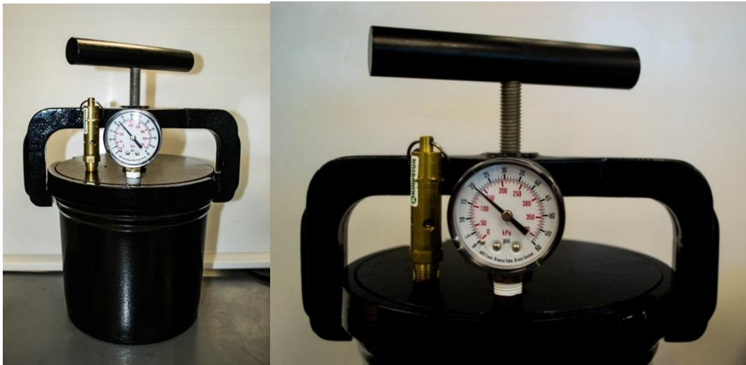
Figure 21 Left: Locked de-pressurizer with samples placed inside. Right: Gage set at ~20psi for ~24 hours.
