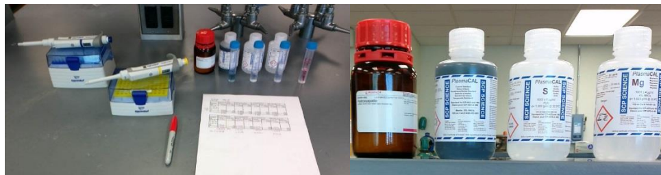
Figure 24 Left: Materials used for creating standard solutions. Right: Pictured from left to right: Synthetic hydroxyapatite, multi-element, sulfur, magnesium.
