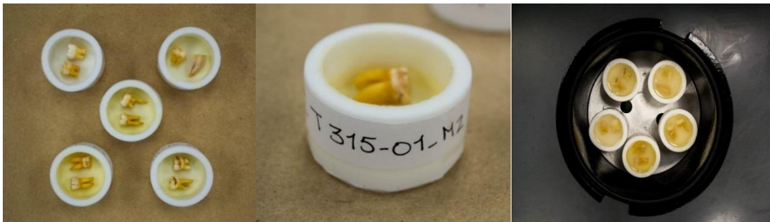
Figure 20 Embedding process. Left: Sample placement in silicone mold prior to resin added. Center: Labelling system used (sample IIT 315-01_M2). Right: Sample placement inside the de-pressurizer chamber.
