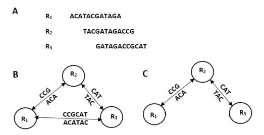
Figure 3.1: Simple string graph representation for three reads. (A) shows three overlapping reads  $R_1, R_2, R_3$ . (B) shows the overlap graph constructed from these reads. Since  $(R_1, R_3)$  is transitive, this edge is not be present in string graph shown in (C).
