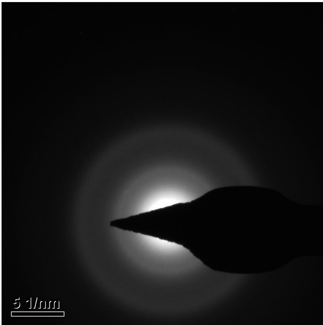
Figure 7: Selected area electron diffraction (SAED) image during HR-TEM of CuSiNG 4 showing amorphous nature of the silica matrix.
