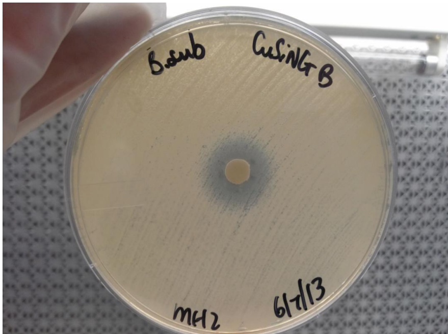
Figure 24- Clear zone of inhibition of ~ 17mm by CuSiNG B against B.subtilis
