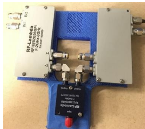
Figure 3.12: Power divider and 180° hybrids.
