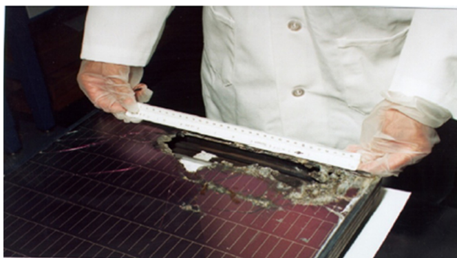
Fig. 4 Arcing and molten glass as a result of corrosion reaching the junction box left a \sim 7 in. long gaping hole, large enough to pass a fist through.
