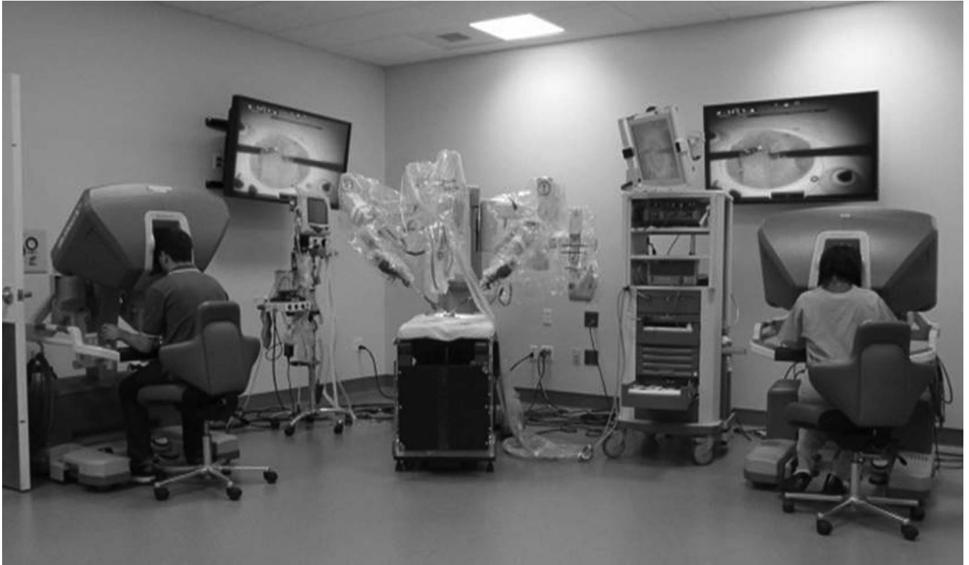
Figure 1. da Vinci Si dual console in use. The surgeon consoles on the left and right both control the robotic arms in the center of the picture.
