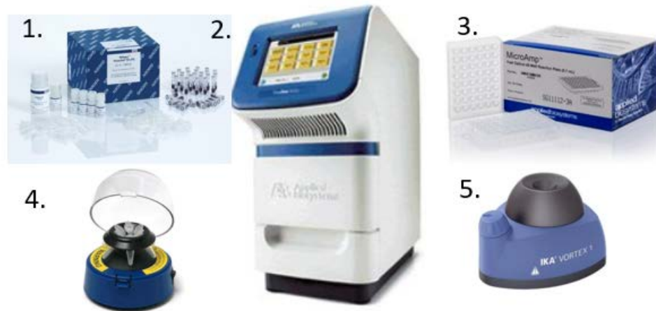
Figure 22 qPCR instrument and Accessories used in UCF Lab (1. DNeasy PowerSoil kit, 2. Applied Biosystem StepOne Real-Time PCR System, 3. PCR 48-well plate, 4. Centrifuge, 5. Vortex mixer)
