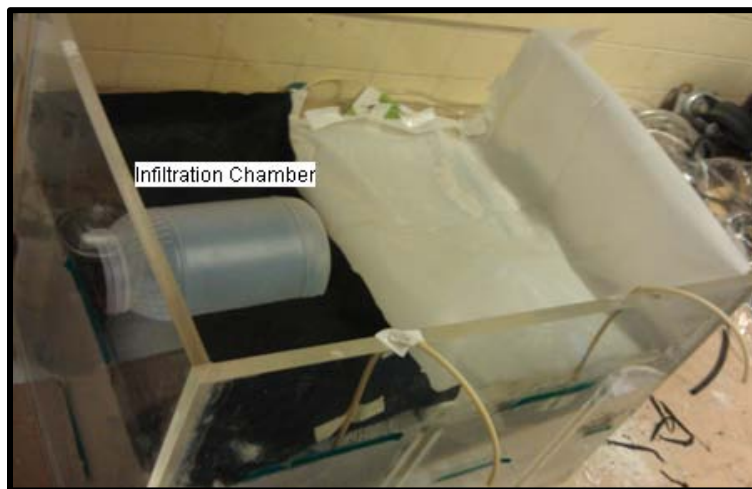
Figure 10 Infiltration Chamber and Impermeable Membrane
