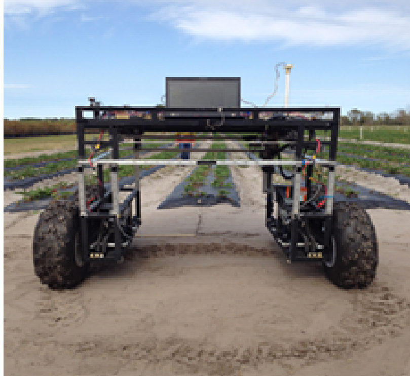
Figure 5.13: DDAGR orientation after a cross-bed motion, desired row is visible appearing at the center of the vehicle in the picture [54]
