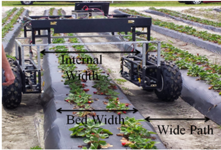
Figure 5.1: Strawberry orchard tests with large travel path widths, DDAGR in its expanded form
