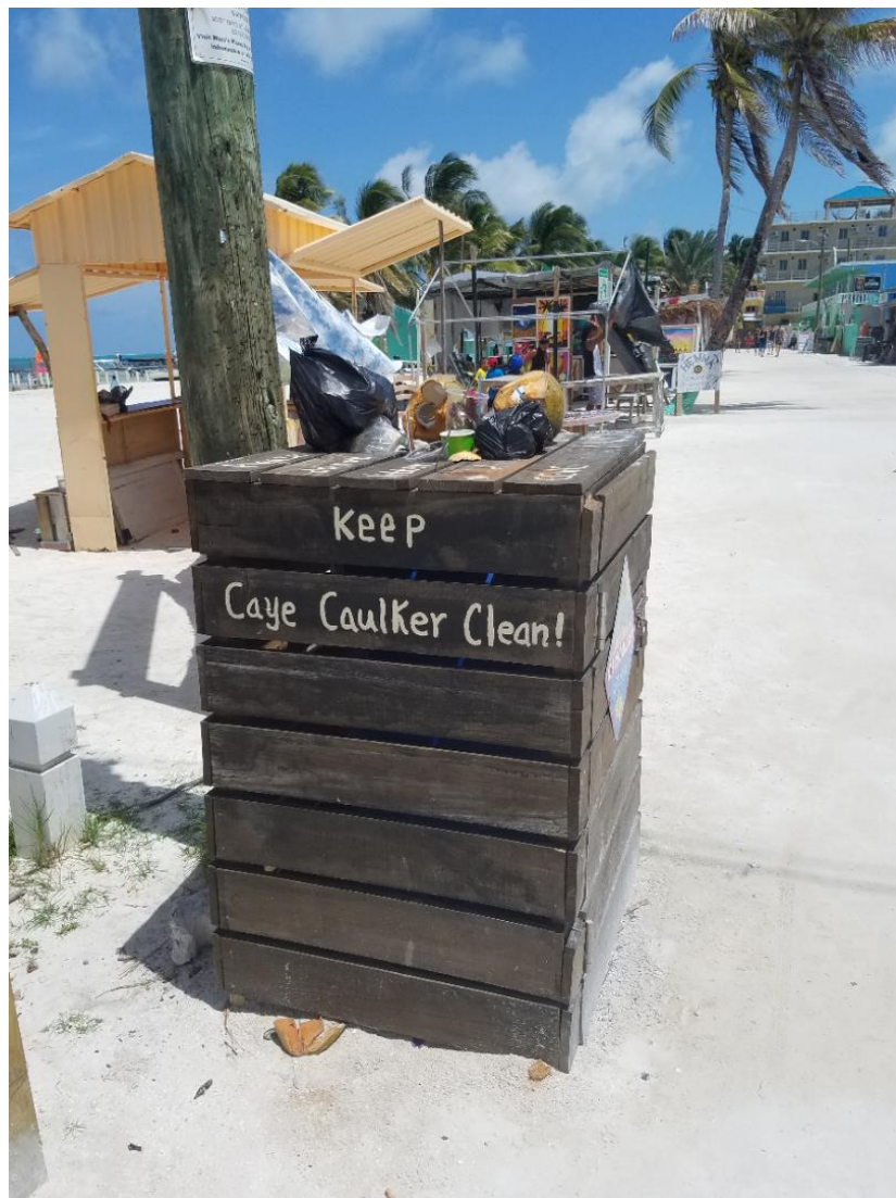
Figure 4: One of the government owned trash cans in the commercial district. Notice the small openings at the top to insert trash and to prevent household garbage bags from being deposited. Photo: Deven Gray
