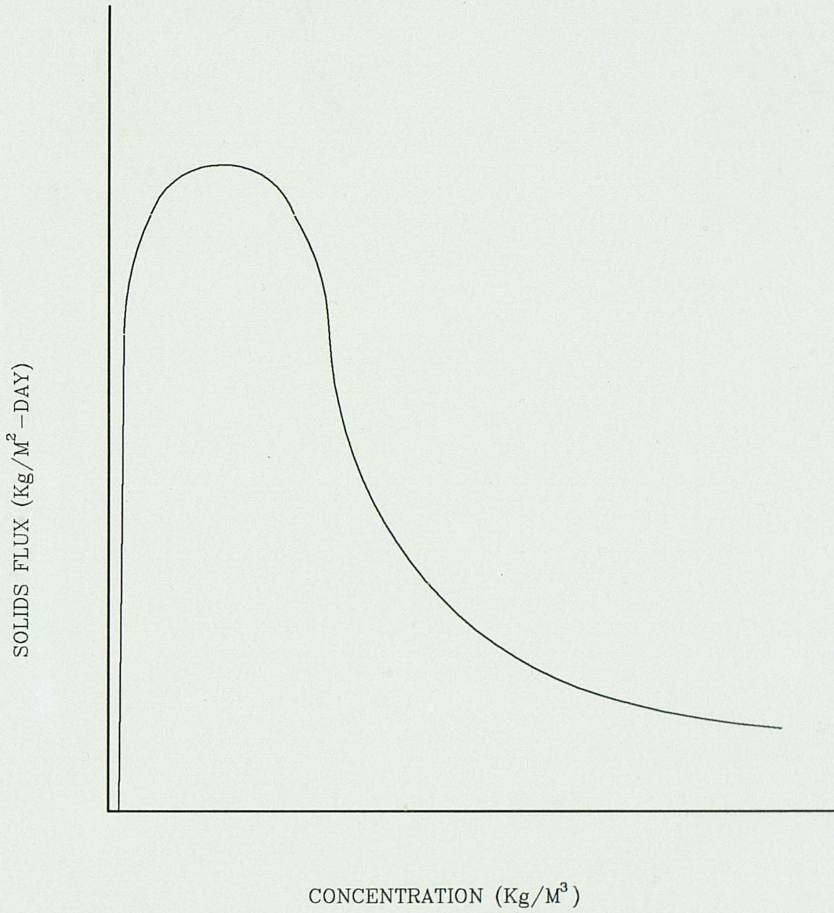
Figure 10. Solids Flux Versus Concentration
