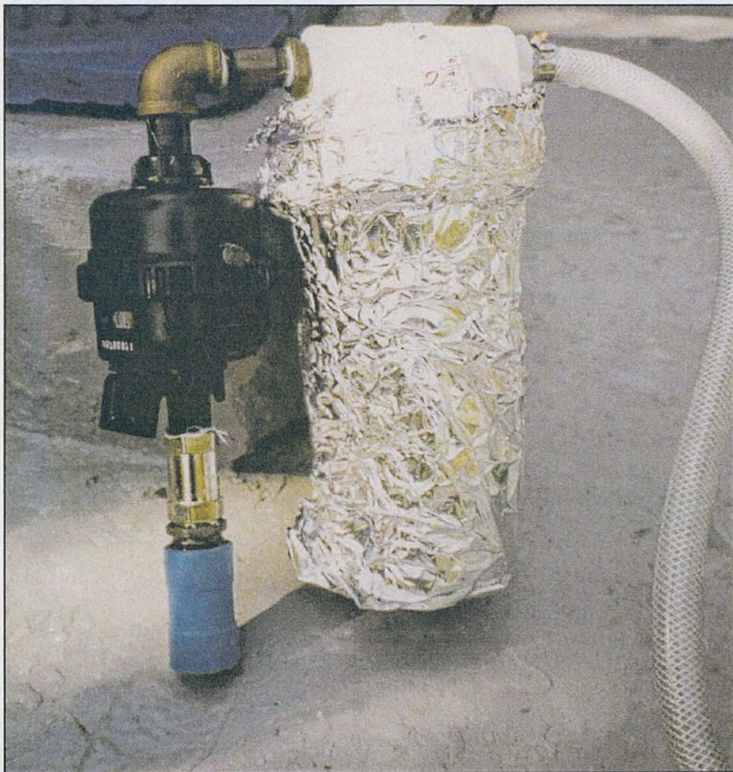
Figure 3.3 Photograph of Water Well Sampling Device
