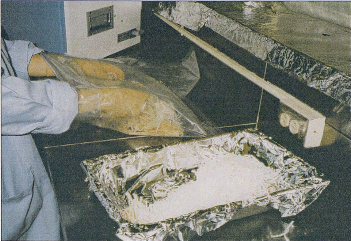
Figure 3.4 Photograph of MPA filter fibers removed from sample spool
