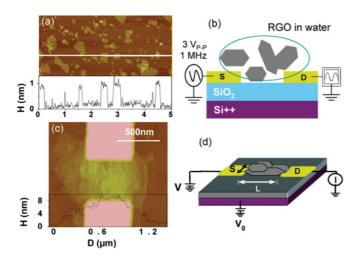
FIG. 1. (Color online) (a) Tapping-mode AFM images of RGO sheets with a height profile indicating the majority of the sheets are single layer. (b) Cartoon of DEP assembly setup. (c) Tapping-mode AFM of a RGO device assembled via DEP along with their height profile. The height (H) varies from 2 to 10 nm in the channel, indicating that up to 10 layers of RGO sheets have been assembled in the channel. Scale bar = 500 nm. (d) Cartoon of electronic transport measurement setup.
