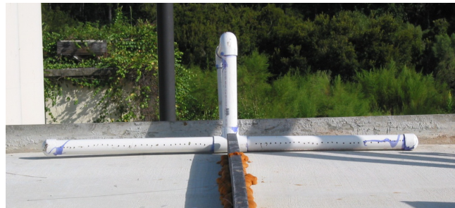
Figure 4. PVC piping system used to create sheet flow over simulated roadway.
