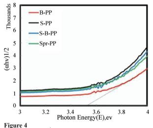
A Plot of  $(\alpha hv)^2$  Versus Incident Photon Energy of PEDOT: PSS Films
