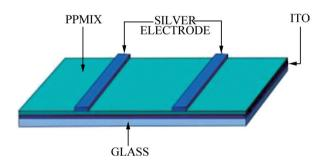
Figure 1 A Schematic Structure of the Device (Ag/PEDOT: PSS/ ITO)
