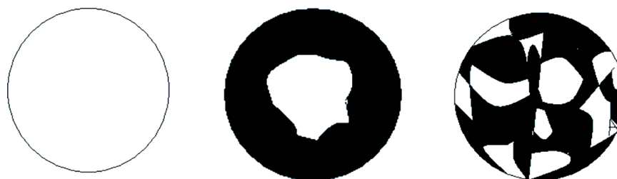
Figure 5 Different Pore Structures of Catalyst (a) Pore of Fresh Catalyst (b) Pore of Normal Deposition (c) Pore-Making in Catalyst Pore
