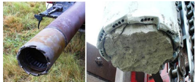
Figure 2 Air Flush Core Barrel and Core Inside the Barrel
