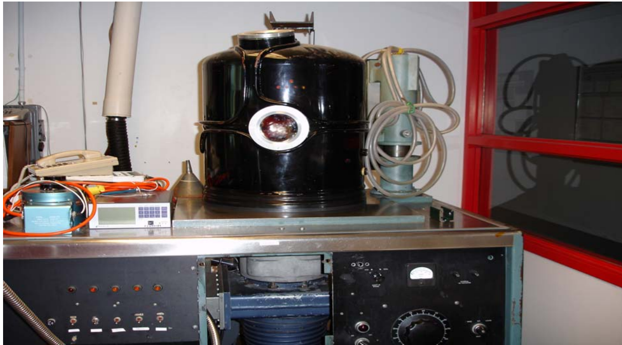
Figure 17 : Thermal evaporation setup.
