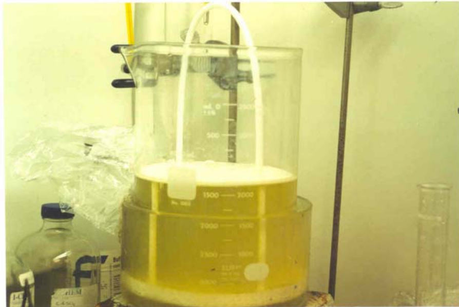
Figure 16 : Set-up for the Chemical Bath Deposition.
