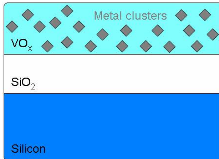
Figure 4.4 Metal Additions to Amorphous \text{VO}_x Thin Film.
