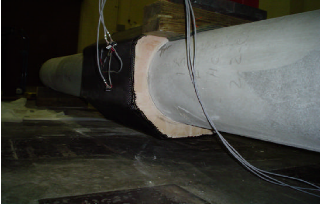
Figure 31: The support near the joint was removed
