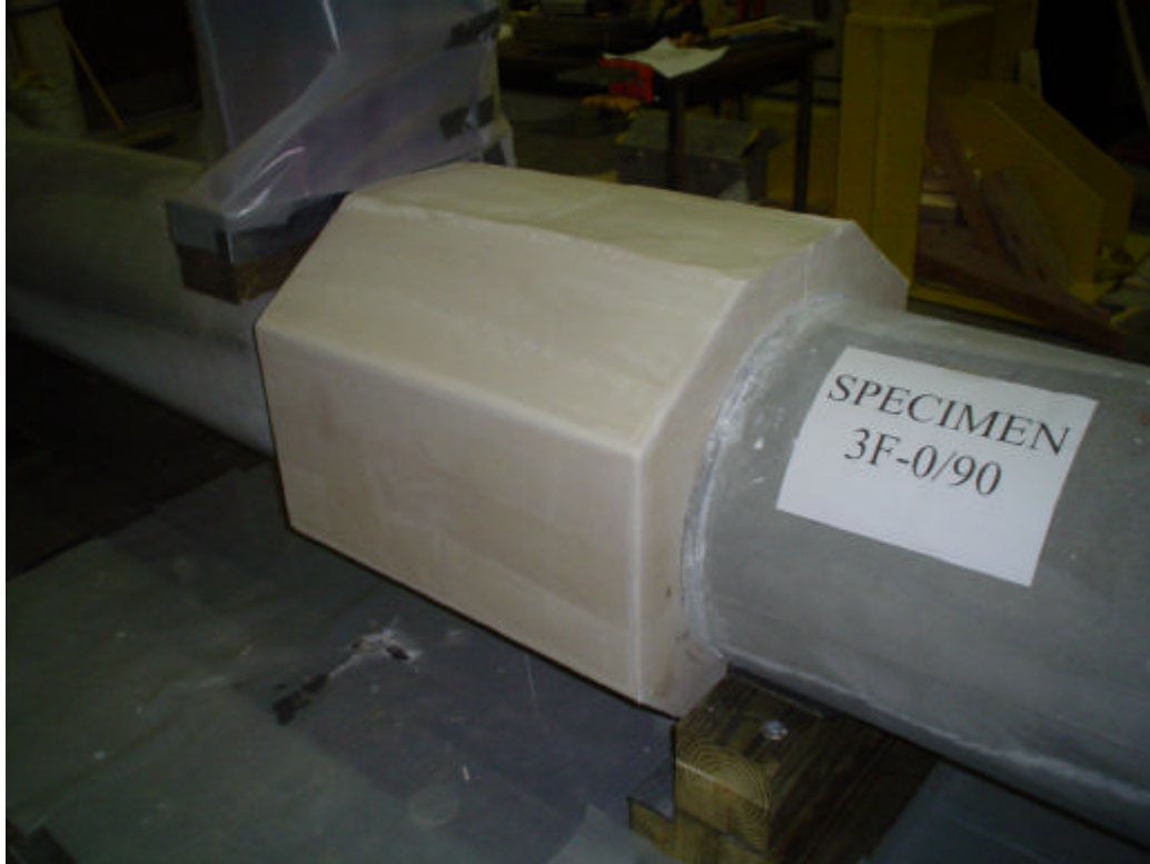
Figure 14: Hydro-Stone rim around pipe joint
