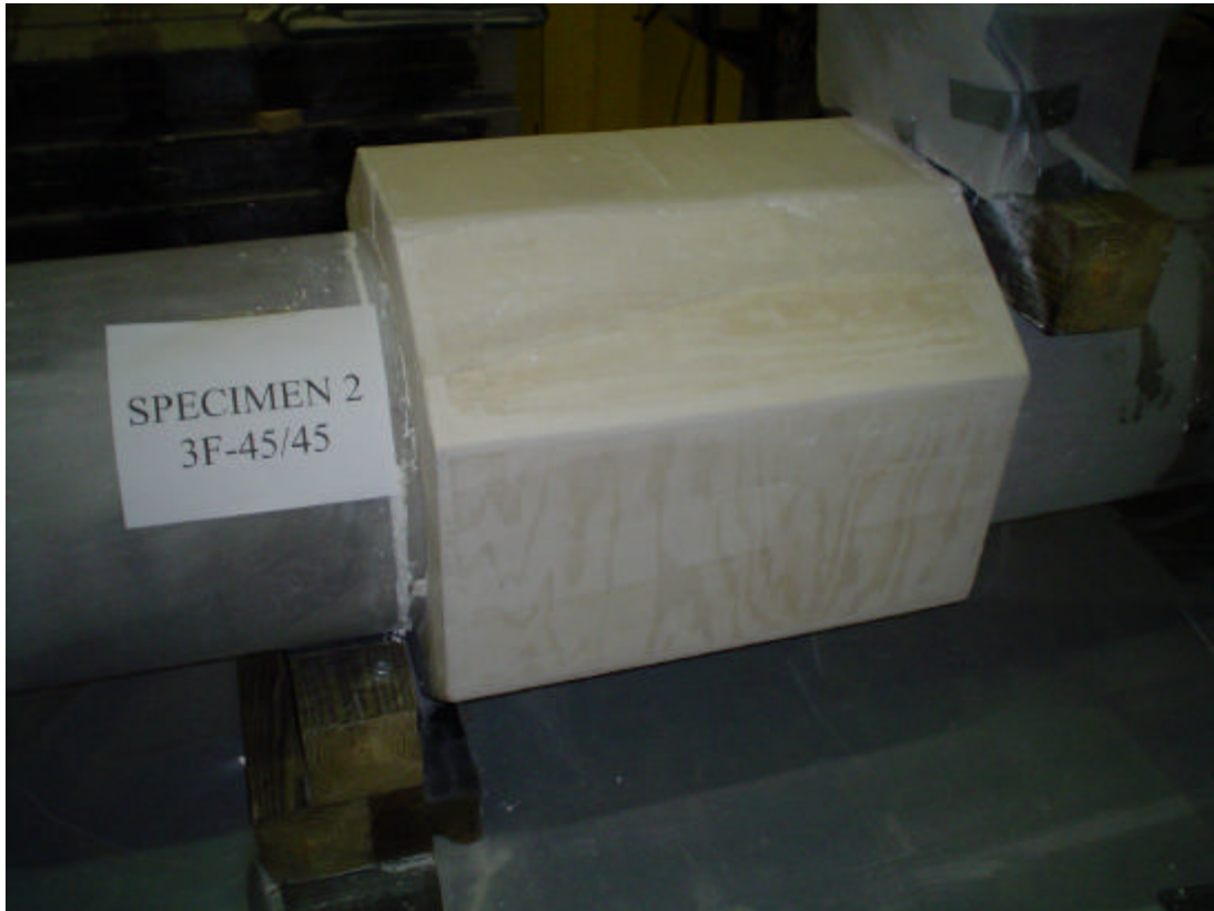
Figure 24: Hydro-stone rim around the joint
