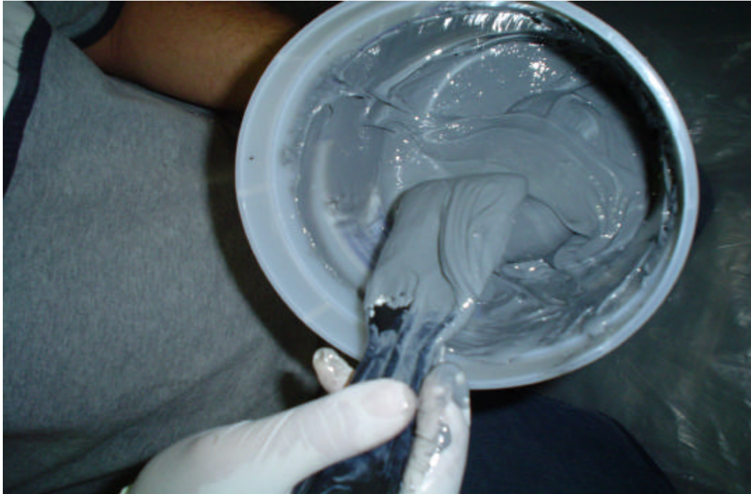
Figure 18: Mixing of QuakeBond J200TC
