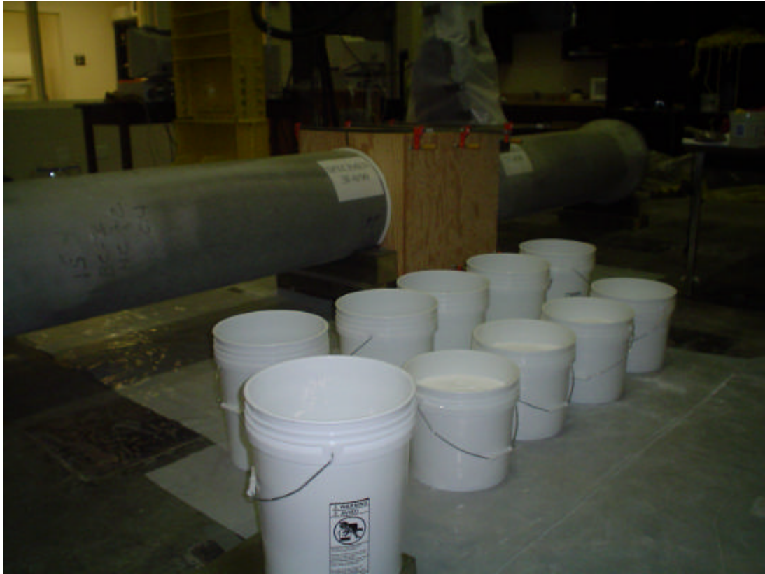
Figure 15: Mixing of the Hydro-Stone in a batch process
