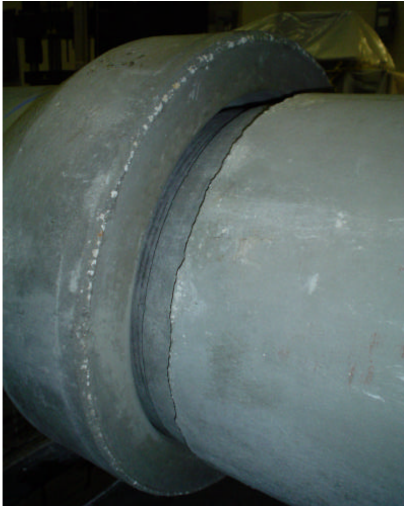
Figure 20: Displacement of the spigot from its regular position
