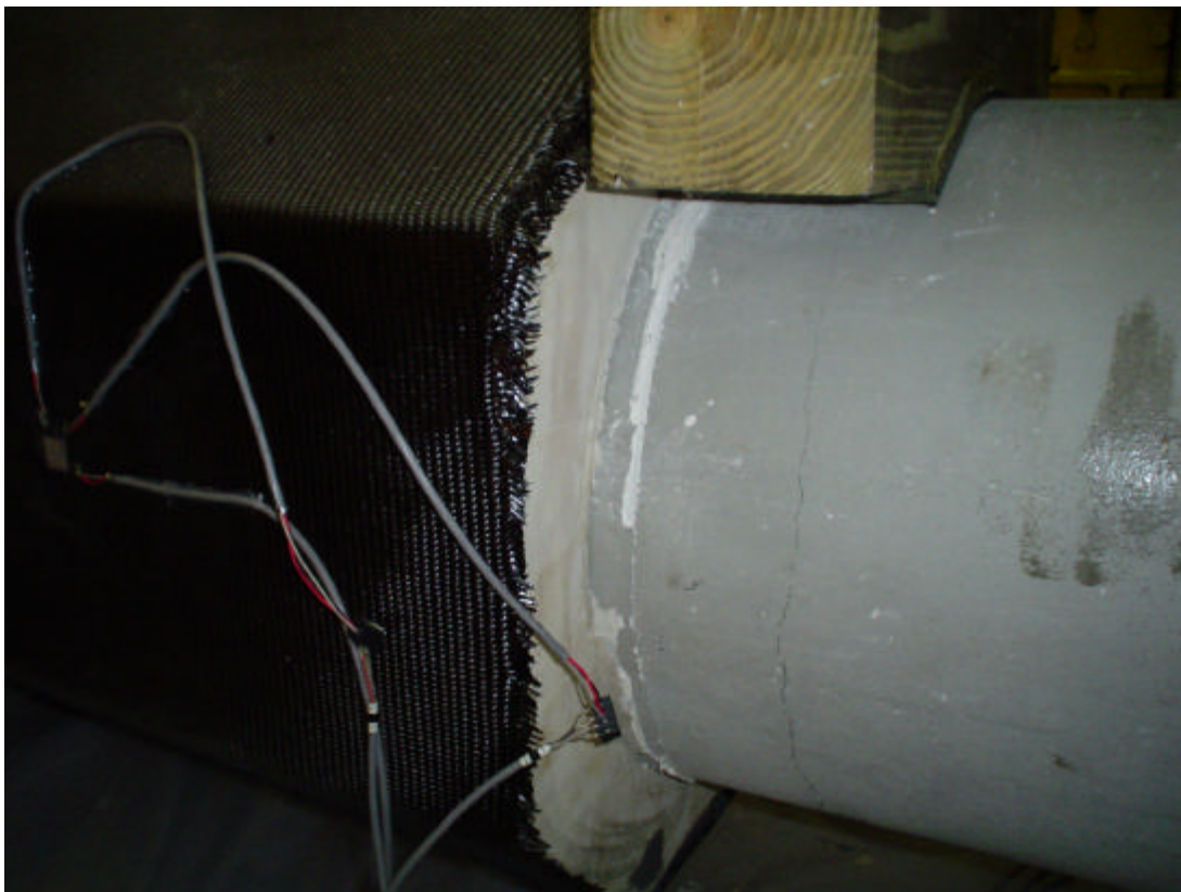
Figure 35: Failure Mode of Specimen 3F-45/45
