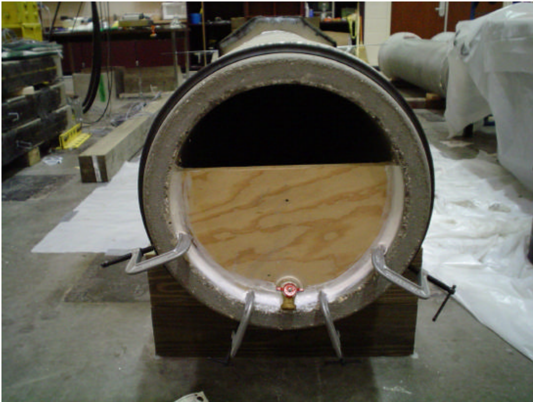
Figure 26: Capping of pipe ends
