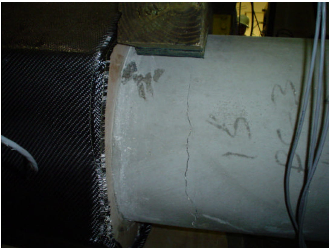
Figure 33: Mode of failure for Specimen 3F-0/90 after removing center support
