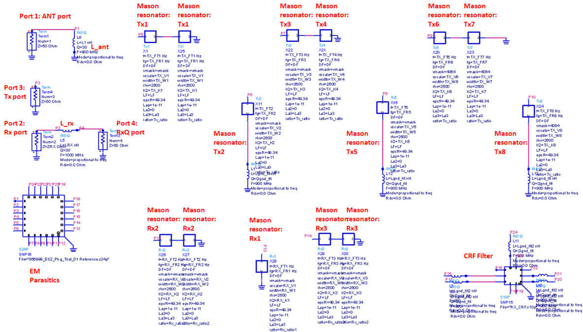
Figure 5-12 Schematic of a WCDMA Band 5 duplexer simulation in ADS.
