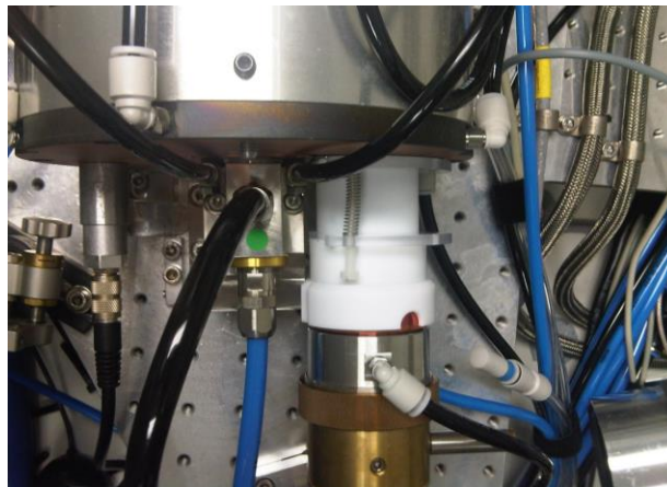
Figure 56: Pump light fed into the back of the pump cavity (disk assembly) via the homogenizer
