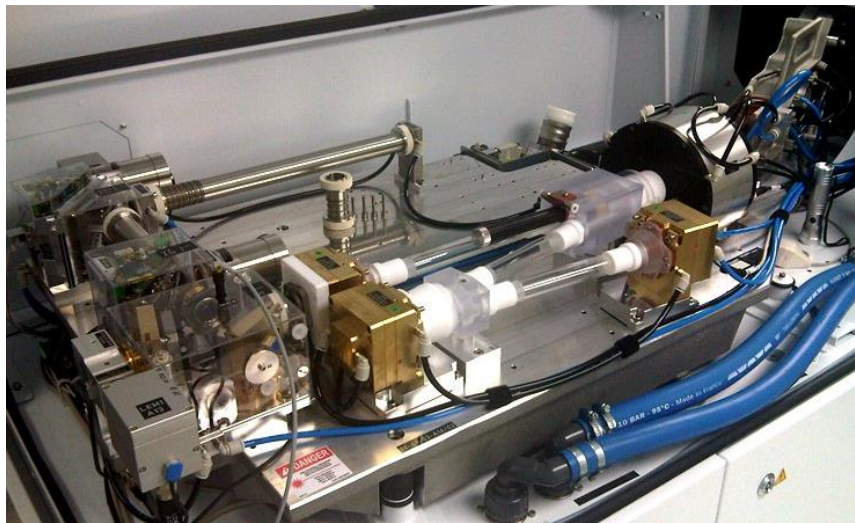
Figure 50: TruDisk 1000 laser cavity as factory installed
