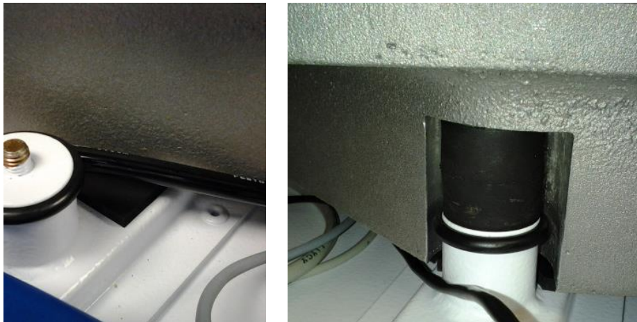
Figure 112: Rubber insulation between the TruDisk 1000 table and the case housing the electronics and cooling system, for damping of mechanical vibrations
