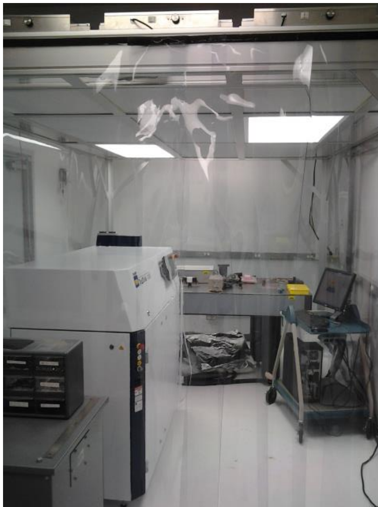
Figure 63: TruDisk 1000 Installed in Class 10,000 Cleanroom
