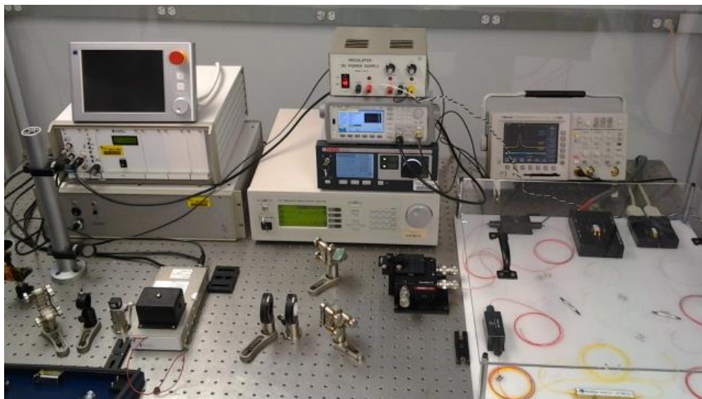
Figure 46: Alternate view of fiber oscillator and pulse picking set-up
