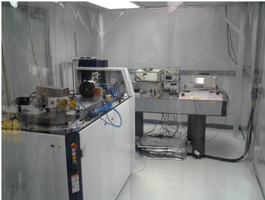
Figure 62: TruDisk 1000 after removal of the factory installed opto-mechanics and container lid housed in the modular clean space
