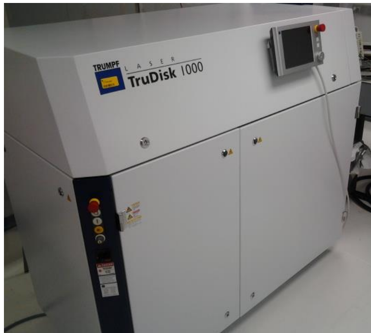
Figure 48: Trumpf TruDisk 1000: 1 kW CW thin-disk laser system
