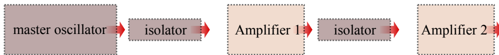
Figure 2.5: Concept of a MOPA. Isolators prevent feedback to the oscillator or pre-amplifiers
