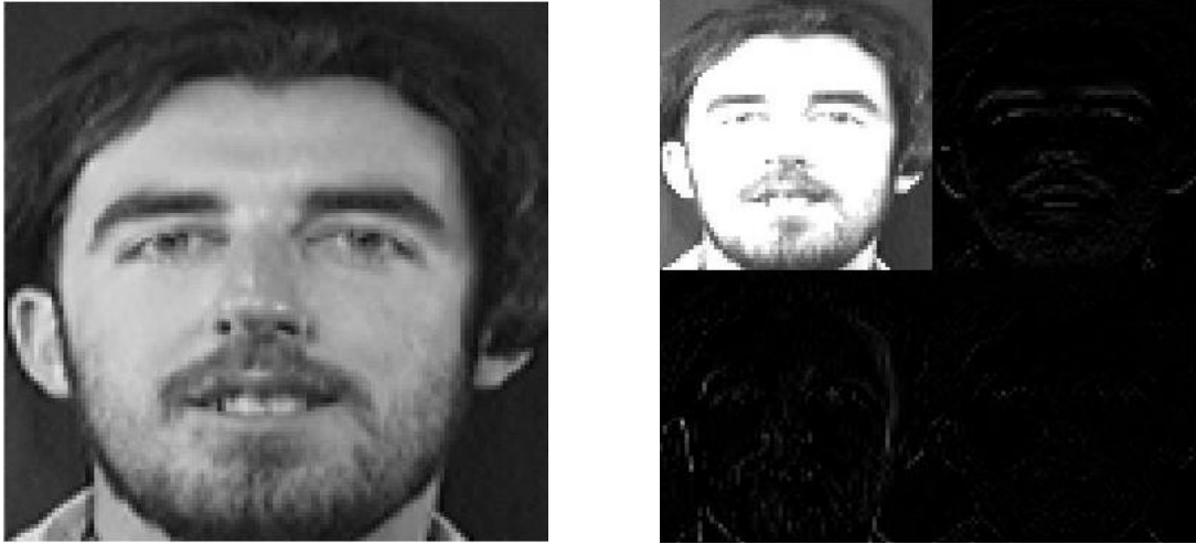
Figure 3.2: Original image (left) and its One-level of decomposition using the Haar function (right)
