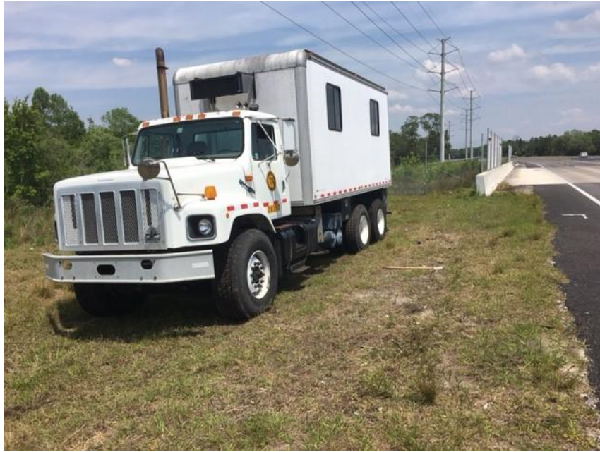
Figure A1: Cone Penetration Test Rig on SR 415
