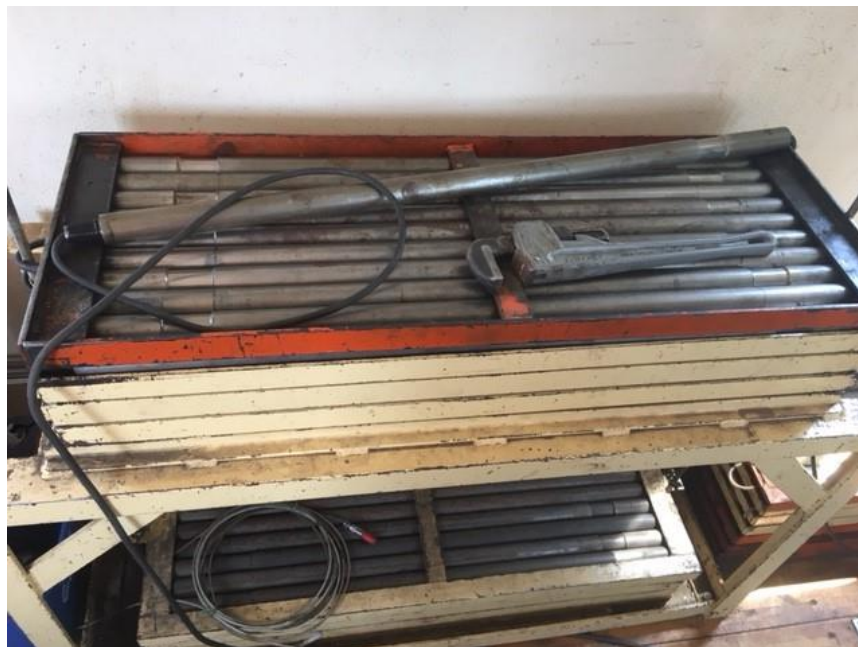
Figure A2: Cone Penetration Test Push Rods
