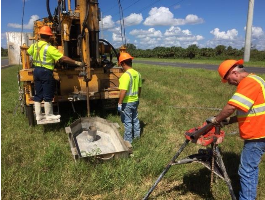
Figure A6: Sample Collection from SPT Test
