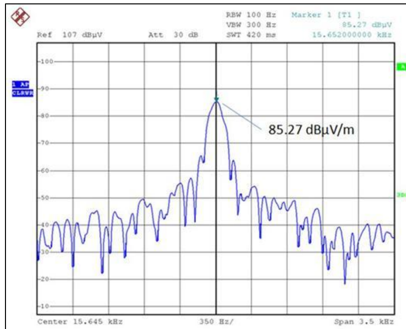
Figure 50: WPT J1 prototype RE-102 (electric field intensity) test setup
