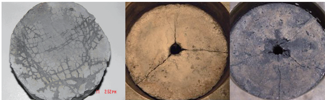
Figure 2 Photos of Rock Damage and Fracture Effect by Exploding
