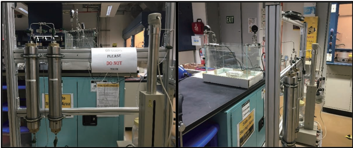
Figure 4 Actual Workstation/Dosing System
