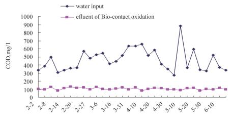
Operation time,month,day Figure 3 The Removal Effects of COD by the Biological Contact Oxidation Process During Stable Operation
