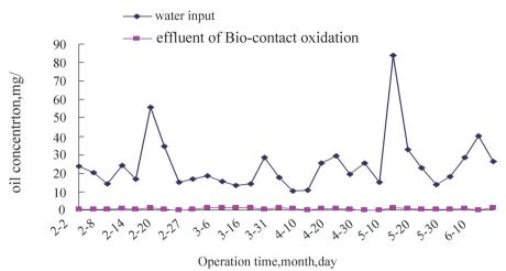
Figure 2 The Removal Effects of Oil by the Biological Contact Oxidation Process During Stable Operation
