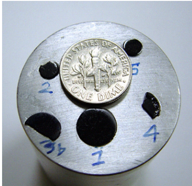
Figure 7-1: CNT-polymer derived ceramic composite specimens subjected to instrumented nanoindentation.
