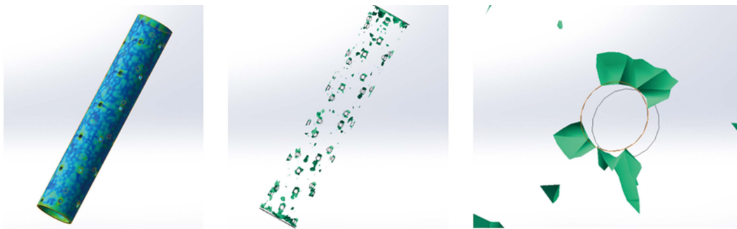
Figure 2 Perforated Casing ISO Tailoring 120 MPa Stress Nephogram
