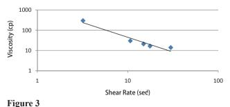
Polymer Solution Viscosity Versus Shear Rate
