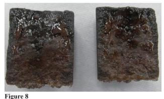
Opened Fracture Showing the Gel Distribution Within the Fracture
