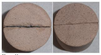
Figure 11 Fractures in the Inlet Side (left) and the Outlet Side (right) for Experiment P2
