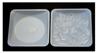
Figure 4 Volumes of Gel Particles Before (left) and After (right) Contacting Water
