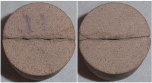
Figure 13 Fractures in the Inlet Side (left) and the Outlet Side (right) for Experiment P2
