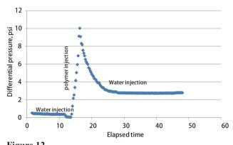
Figure 12 Different Pressure During Water-Polymer-Water Injection for Experiment P2
