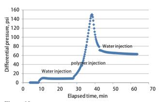
Figure 10 Different Pressure During Water-Polymer-Water Injection for Experiment P1
