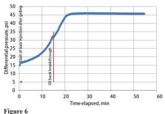
Pressure Changes During Waterflooding After Particles Swollen
