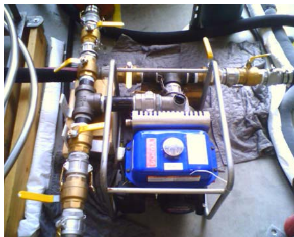
Figure 9. Yamaha Pump, 123cc, 4-stroke gasoline driven
