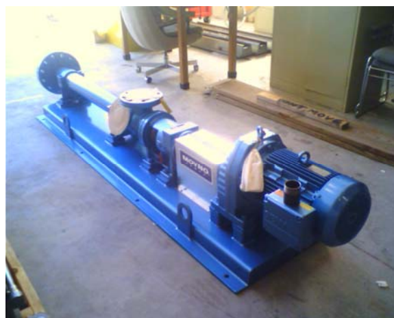
Figure 10. Multi-Phase Pump 4-stage, 15HP
